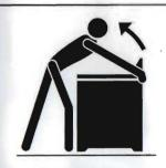
To check if the anti-tip bracket is installed properly, use both arms and grasp the rear edge of range back. Carefully attempt to tilt range forward. When properly installed, the range should not tilt forward.
